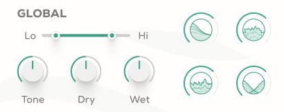
Lo: Cut out frequencies from the wet signal below the set frequency.
